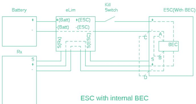
The red and black power cables (10 AWG) marked “BAT” should be connected directly to the battery supply.
